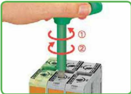
... A small counter-clockwise rotation releases the latch ①. Once the hex wrench ② has been removed, the conductor is clamped safely.
