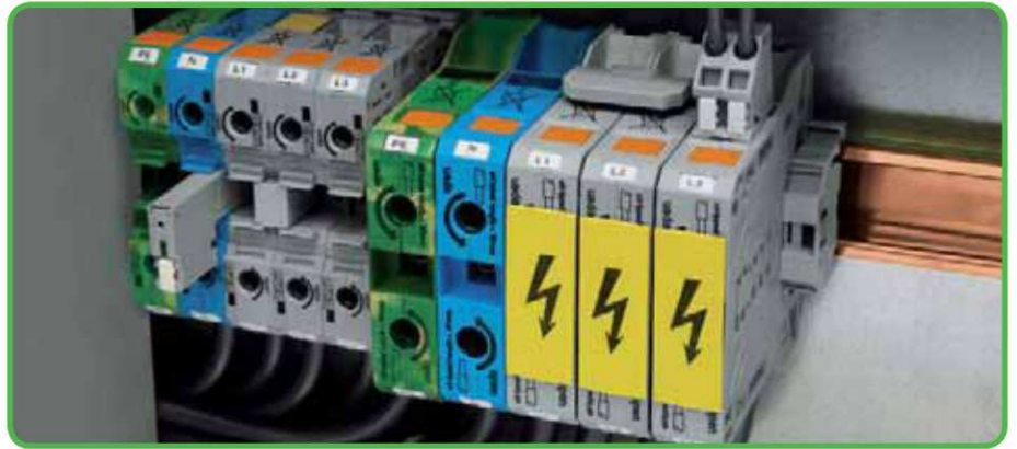
Insert stripped conductor (stripped length 35 mm/ 1.38 in!) into the clamping unit until it hits the stop; hold conductor in position ...
