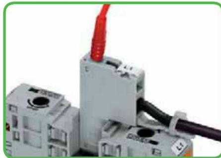
The voltage tap is inserted into the jumper contact slot. It can be fitted with a strain relief plate and provides test option for Ø 2 mm/0.079 in test sockets.
