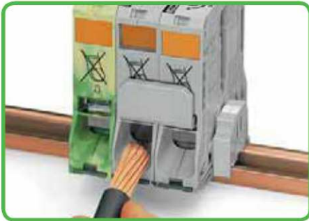
Insert stripped conductor (stripped length 35 mm/ 1.38 in!) into the clamping unit until it hits the stop; hold conductor in position ...
