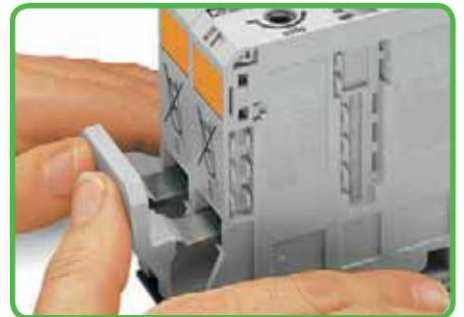
Commoning with adjacent jumper. Insertion of jumper above the conductor entry hole, without tools. Rated cross section is still 50 mm 2 /AWG 2/0 and 95 mm 2 /AWG 4/0.
